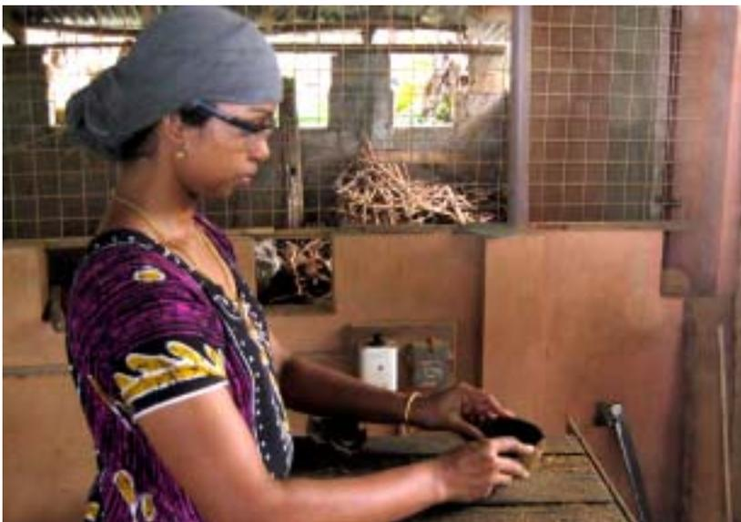
*Cutting the shell to the required shape*
